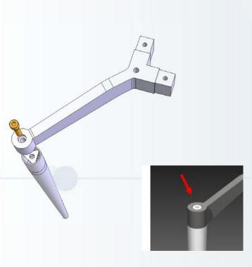
Only one screw for fixing arm and leg!
