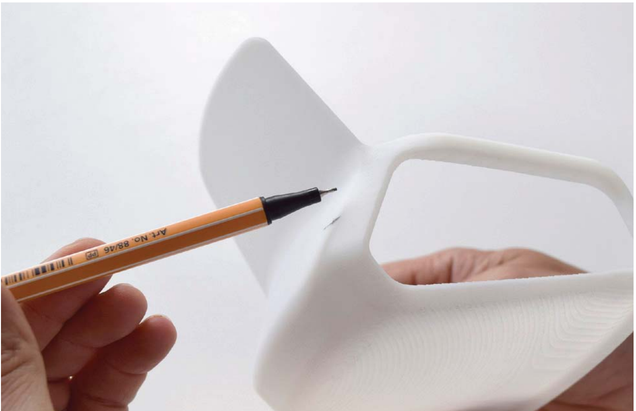
Despite all the hard work done on the computer during the design and development phase, its aesthetic was enhanced based on models produced as 3D-printed objects during a laser sintering process.
