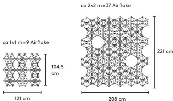
Note! Depending on how the modules are assembled, the total measurement differs.
