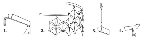
1. Skena/rail/Schiene (L:1500, 2000, 3000 mm)
